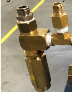
IBEX: Where to locate pressure transducer underneath pump.
