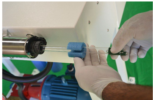
Figure 2. Lamp placed into filter housing.
