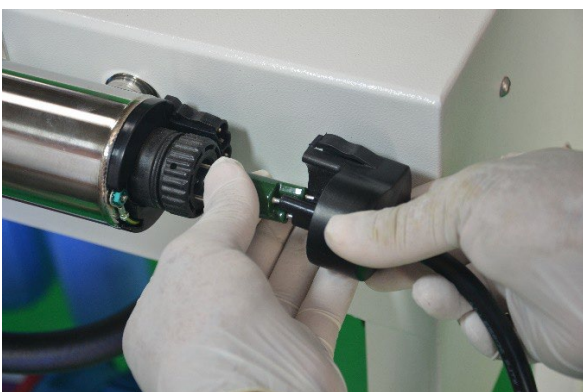
Figure 3. Lamp plugs into receptacle. 2-Piece Filter Housing clicks into place.
