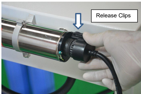
Figure 1. Push clips on filter housing to release the bulb receptacle (top).
