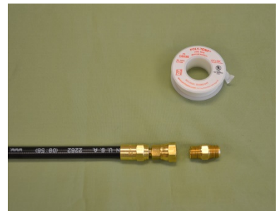
Figure 12: Female Swivel Fittings Do NOT Require Tape on the Male Fitting
