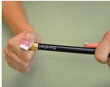
Figure 2: Screw Ferrule onto Hose Counter/Anti Clockwise
