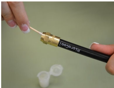
Figure 7: Apply Silicone to Inside of Ferrule
