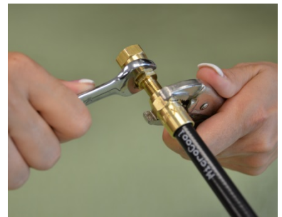
Figure 9: Using a Wrench, Screw in the Ferrule
