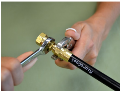
Figure 10: Stop with 1/8" - 3mm Gap
